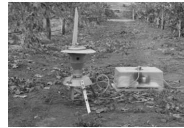
Fig. 4: Volumetric spore trap. [1]
